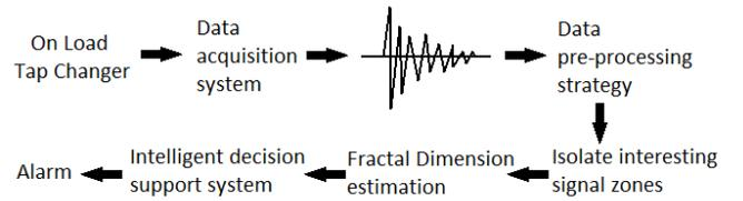
Fig. 3. Schematic representation of the proposed diagnostic system
