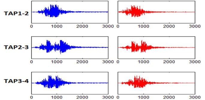
Fig. 8. Vibration fingerprints for TAP positions 1-4 with different accelerometer mounting methods
