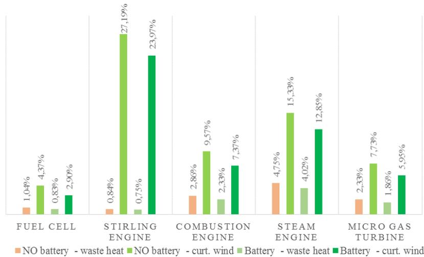
Fig. 5. Unused energy amounts for microgrid with and without the battery storage (in percent to total heat used || total wind energy production)
